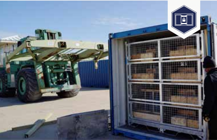
Move the SHARKCAGE into standard containers The SHARKCAGES are designed to be transported in standard shipping containers, TRICONs or on air pallets. Move directly into the container using a forklift and you are ready to move.
