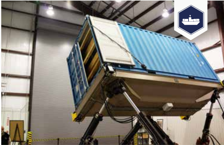
Transport using any mode of transport Testing at Defense Ammunition Center in McAlester (DAC) has proven the cages are strong enough for any mode of transport, even when fully loaded with ammunition.
